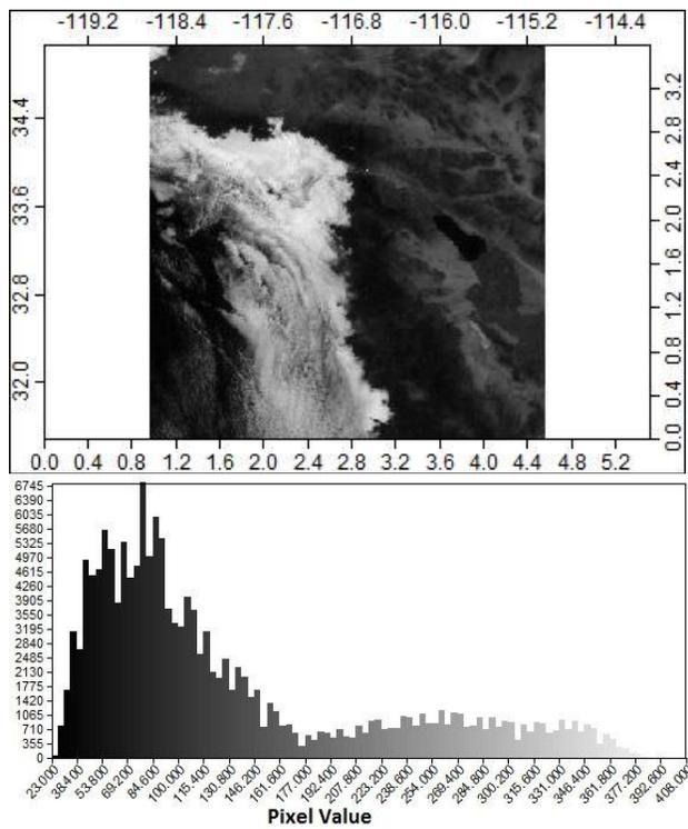
Fig. 1. Example histogram for VIS spectrum images showing two distributions of pixel frequency corresponding to bare ground (left peak) and cloud cover (right peak).
